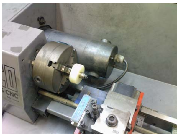
Figure 2. The lathe and the workpiece clamped
