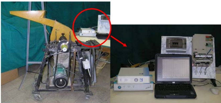
Figure 2. Zenit Junior hammer mill and the measuring system SPIDER 8 data recorder, Measurement Computer, Frequency inverter
