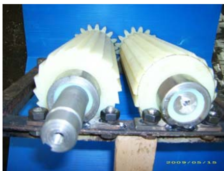
Mill for fruits. Milling drums and gears are made of cast polyamide 6. Original parts were made of steel
