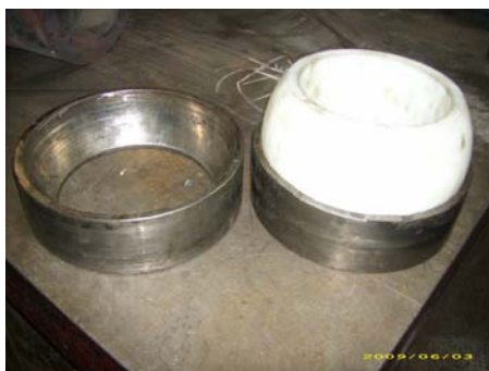
Spherical bushing made of cast polyamide 6. Replacement of fast wearing POM C bushing.
