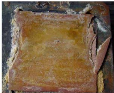
Figure 3. Edge disintegration of a reinforced polymer specimen after large scale friction test.
