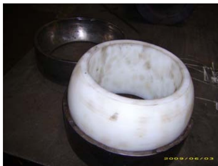
Spherical bushing made of cast polyamide 6. Replacement of fast wearing POM C bushing.
