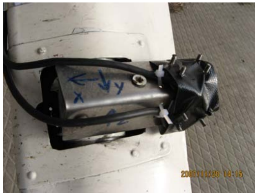
Figure 6. Acceleration sensors on the landing gear leg
