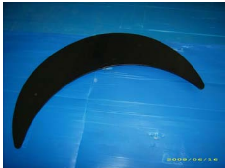
Airport transporting belt: support wear pad, made of UHMW-PE HD 1000. Formerly steel and other polymer was applied.
