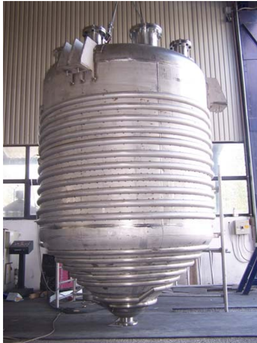
Figure 4. Practical example of half pipe channel
