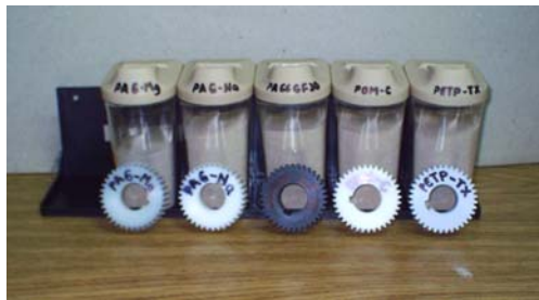
Figure 3. Gears (according to Fellow's technology) with the reference abrasive media (siliceous sand)
