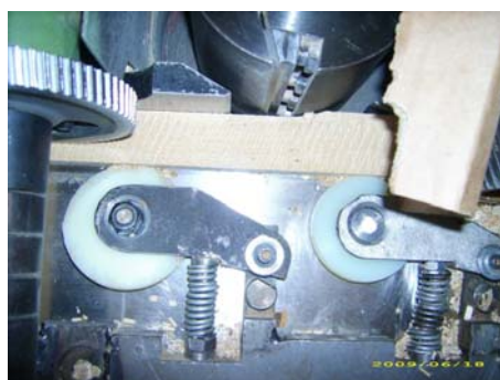
Regulating rollers in wood processing machine, made of cast polyamide 6. Earlier steel was applied.
