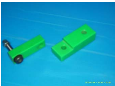
UHMW-PE HD 500 material, a part of bread slicer. Originally CrNi steel was applied.
