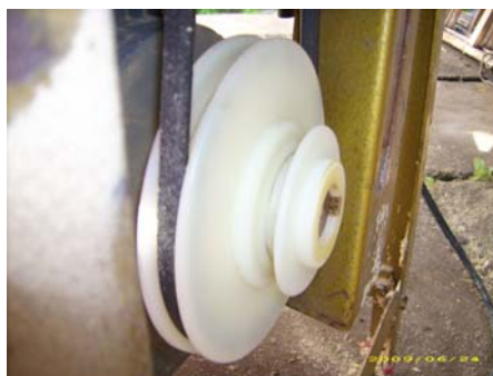
Cast polyamide 6 V-belt pulley for circular saw. Earlier steel was used.
