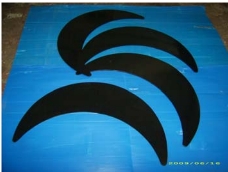
Airport transporting belt: support wear pad, made of UHMW-PE HD 1000. Formerly steel and other polymer was applied.
