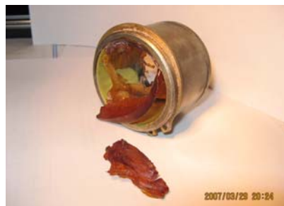
Figure 4. The failed PUR component
