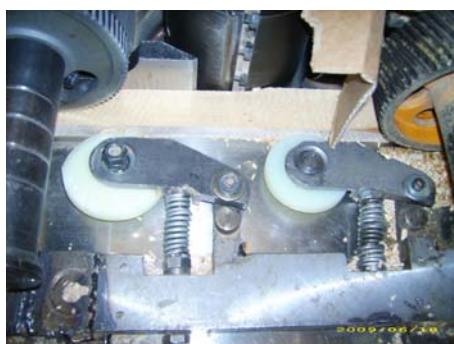
Regulating rollers in wood processing machine, made of cast polyamide 6. Earlier steel was applied.
