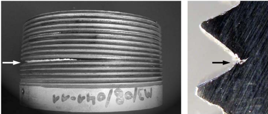
Figure 8. a) Fatigue crack emanating from LET pin, b) detail of the root of the LET of the pin.
