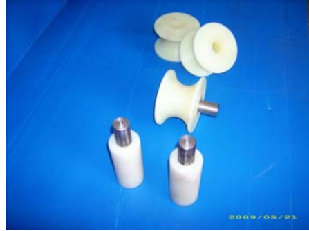
Cast polyamide 6 rollers of moving gates. Originally steel was applied.
