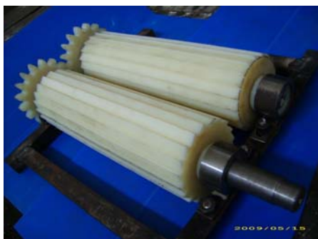
Mill for fruits. Milling drums and gears are made of cast polyamide 6. Original parts were made of steel
