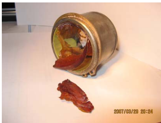
Figure 7. The failed PUR component
