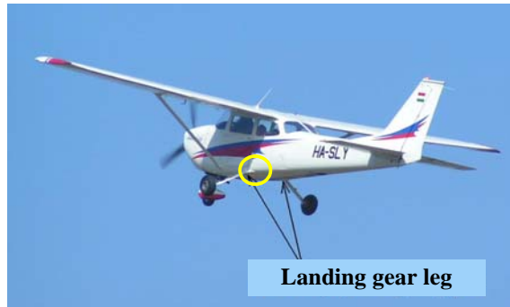
Figure 2. Position of landing gear leg on Cessna 172 type aircraft
